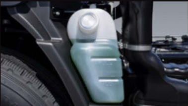
Translucent coolant tank This white, translucent tank makes it easy to check coolant level.
