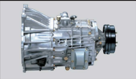
Aluminum transmission case The aluminum pot-type transmission case dissipates heat more efficiently, making this transmission quieter and more durable.
