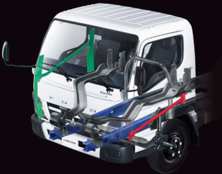
Rigid cab Rigid box and door-well frames, side impact beams, and reinforced cab floor protect all riders in case of collisions.
