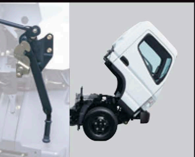
Passenger-side cab tilt lever Allows roadside tilting without standing in traffic.
