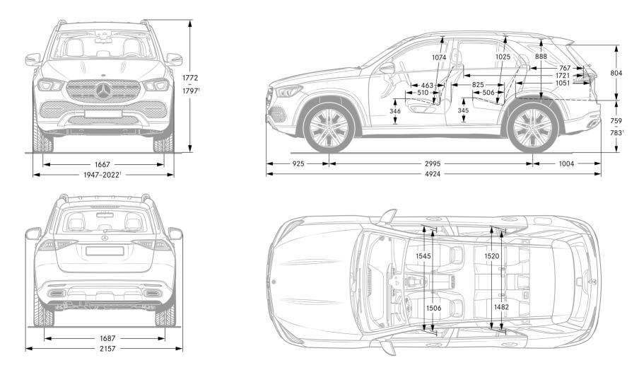
¹ At minimum to maximum height with steel suspension. All figures in millimetres. The illustrated dimensions are mean values. They are valid for vehicles in basic specification and in unladen condition.
