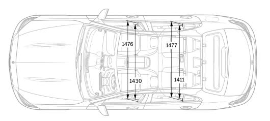
$All\ figures\ in\ millimetres.\ The\ pictured\ dimensions\ are\ mean\ values.\ They\ are\ valid\ for\ vehicles\ with\ standard\ equipment\ and\ in\ unladen\ condition.$
